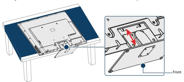
4 Secure the stand column to your TV with the four provided M5  $\times$  12 mm screws (the short screws).
